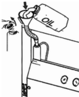
Fig. 135: Filling with oil
