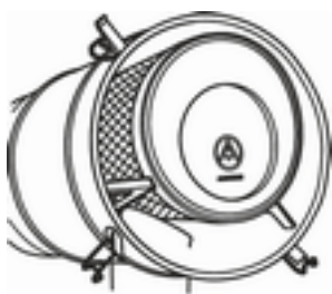
Fig. 31: Opening intake silencer with filter
