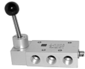
HVR 520 701 L Lever actuated 5/2-way spool valve, indexed. The user can put a padlock through the 5 mm hole of the extended spool and hereby lock the valve. Temperature range: 0°C to 120°C. Seals made from FKM.
