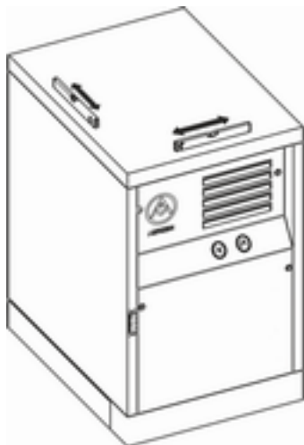
Fig. 54: Spirit level alignment
