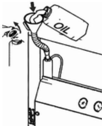
Fig. 106: Filling with oil
