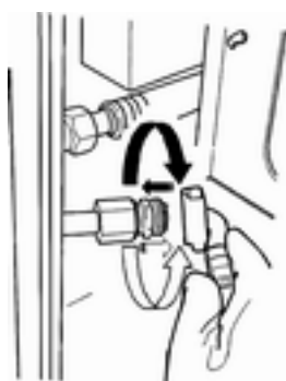
Fig. 121: Fitting the drain hose
