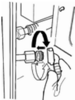
Fig. 134: Fitting the drain hose
